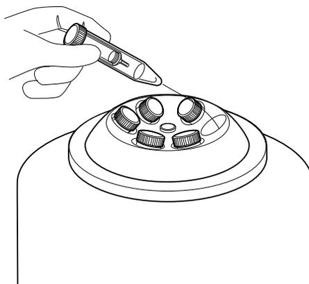
general terms. Forces greater than these numbers may be used, but first examine the effect on analyte recovery. With centrifugation, the disk cartridge is suspended in a test tube and placed into a carrier tray that fits into the centrifuge.
