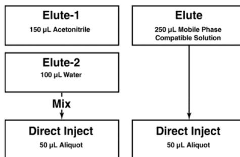
The volumes shown above are only examples. Elution volume will vary depending on the disk cartridge size, the physical/chemical characteristics of the analyte, affinity of the analyte for the chosen sorbent, and the strength of the eluting solvent.
