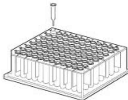
The Empore™ Cat. 610 Vacuum Manifold accepts deep and shallow well collection plates and microtubes. Spacers supplied with the manifold may be used to raise the collection device to the optimal distance below the tips of the disk plate. The illustrations below show that two spacers are used with a deep well plate, no spacers are necessary for the microtubes, and a shallow well plate uses an empty microtube rack as a spacer.
