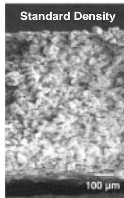
Cross section of a standard density (SD) Empore™ disk (40-60 μm particle size)
