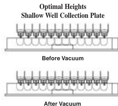
Autoinjectors are commercially available that accept deep and/or shallow well plates. After covering the plate with an appropriate material for sealing, it can be loaded into the injector for analysis, eliminating the need for sample transfer to individual vials. Collection plate manufacturers provide a variety of options to seal plates. The analyst must prioritize the assay needs (evaporation, contamination, freezing, storage, resealable, etc.) and select the appropriate sealing method.
