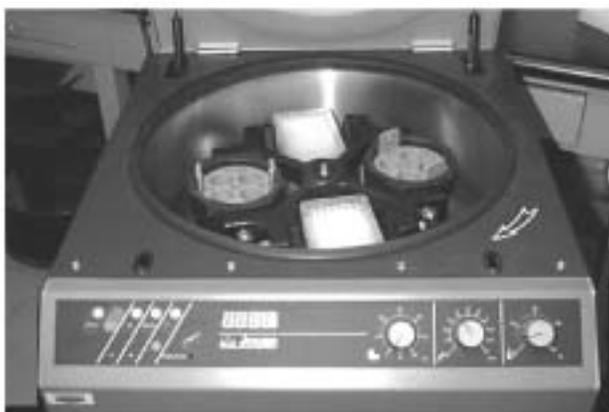
*Centrifugation is an effective method to process liquids through the Empore™ extraction disk plate*
