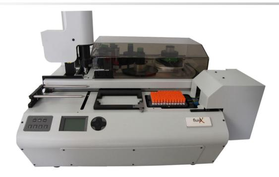
The Xtl-96 is a highly specialised print and apply label applicator for automatic application of individually printed labels on tubes in 24, 48 and 96-format racks.
