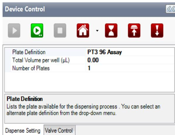
The screenshot shows the 'Device Control' window with a toolbar at the top containing icons for Run, Run with Protocol, Stop, Home, Skip Dispense, Move to Idle Position, Move to Install Chip Position, and Move to Install Input Position. Below the toolbar is a table with the following data:
