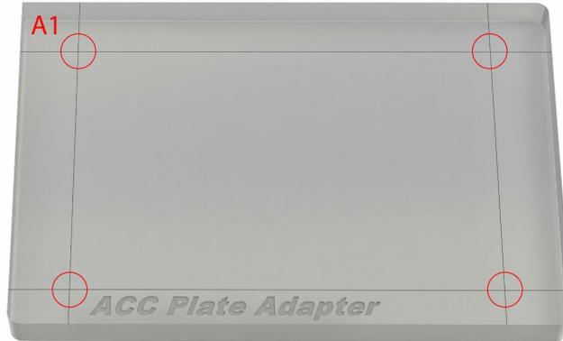
4. Place the reference plate on the Mantis's plate holder. Use the **A1** location (indicated by the red circle) as the reference point.
