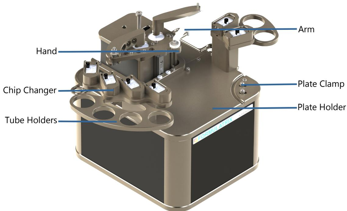
**Arms** The Mantis's arms control the hand movements when dispensing, loading and unloading chips.
