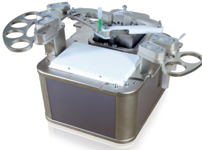
5. Fill the wash container(s) with distilled water and/or wash solution (if you are using wash solution, you must follow the wash solution with a water rinse). Make sure that the wash container(s) contain enough water or wash solution and they are properly placed in the wash stations located at the back sides of the Mantis.
