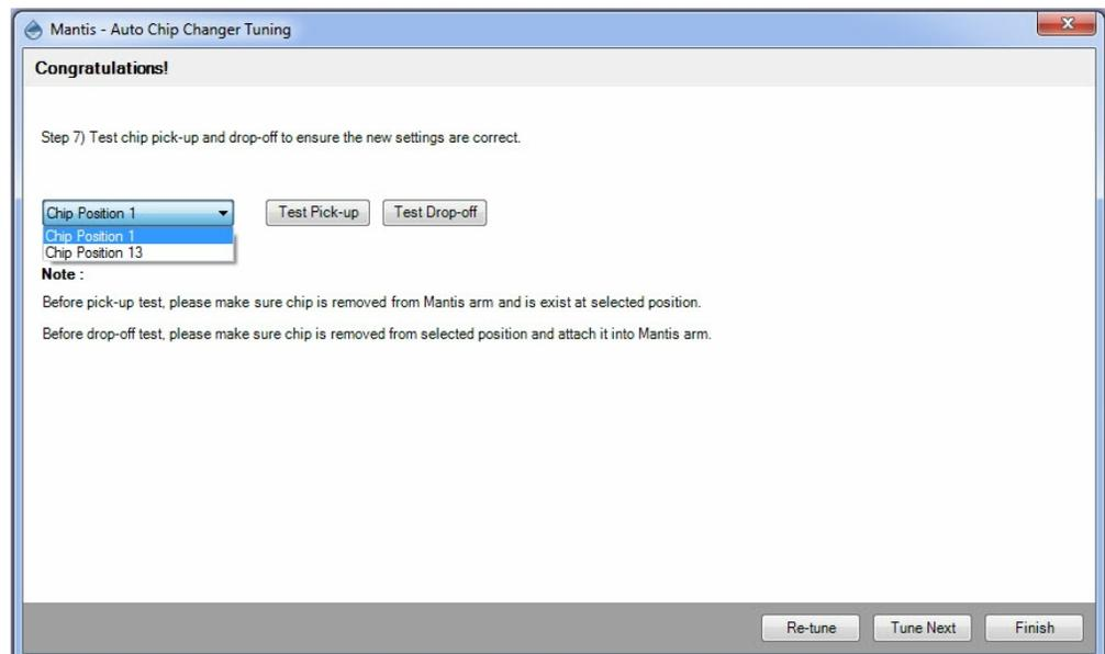
**Note:** If you have the 18 chip carousel, you can test for position 1 and position 10. If you have the 24 chip carousel, you can test for position 1 and position 13.
