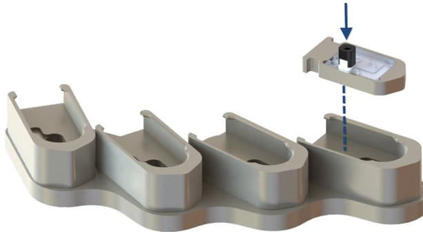
3. Attach the reagent tubes or pipette tips to the ingredient input at each chip. Skip this step if you are using CF chips.
