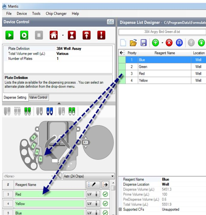
5. Attach your reagents to the Mantis's chips (if you are using pipette tips, you will need to remove the black adapter from the chip's input first).
