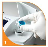
Scan lot calibration barcode. Remove foil from cartridge and insert into analyser.
