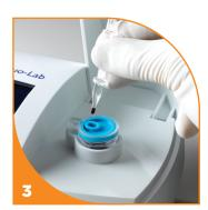
Insert sample tool into cartridge and snap off handle.
