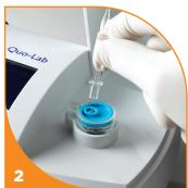
When prompted press reagent bead into cartridge using the reverse end of the sampling tool.
